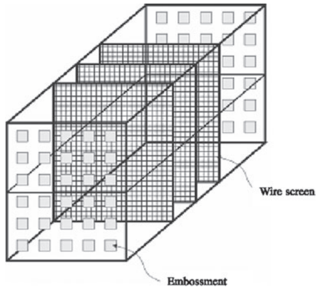
Figure 1. TLD with damping screens (Tait et al. , 2004)
